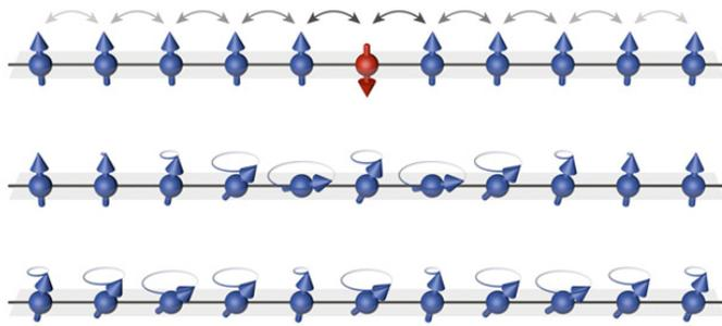
Figure 1: Illustration of the propagation of the spin impurity (red) through a chain of atoms with initially opposite spin.
